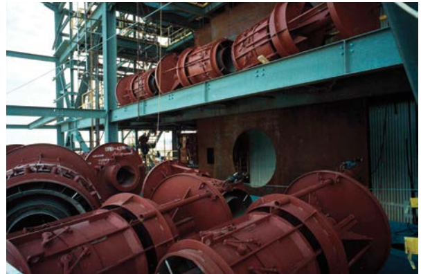
The DRB-4Z burner remains B&W's lowest NO x burner in applications without overfire air systems or where existing boiler geometry is not suitable for use of the AireJet burner.
