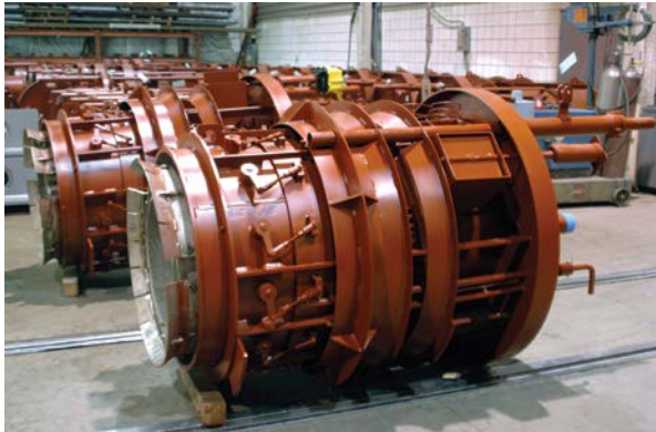
Used with an overfire air system, B&W's AireJet burner provides the ultimate solution for low NO x emissions.
